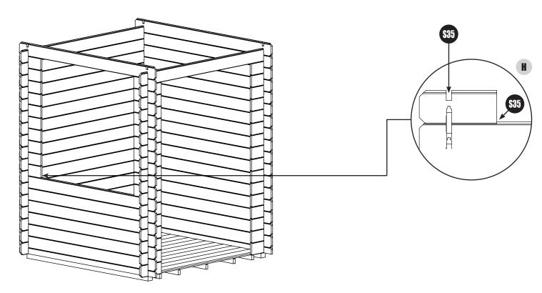
• Install apex gable tops as shown below. Secure into walls using 2x 35mm (\$35) screws per header.
