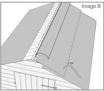
On buildings where a ridge piece is not supplied, roll out the mineral roofing felt along the lower part of one side of the roof. Allow sufficient overhang to fold down on to the roof framing but not the underside of the roof. Use clout nails to tack in to the framing and the upper edge of the felt (Image C). Repeat this on the other side, as long as the felt has not been set too low there should be enough to fold over the ridge, with out the need for extra felt (Image D).
