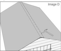
Once the felt is secure, you can cut off any excess and attach the barge boards which will hide any untidy edges and then finish assembly by attaching the finials. Please note bargeboards are only supplied for the gable ends and not the lower edges of the roof.
