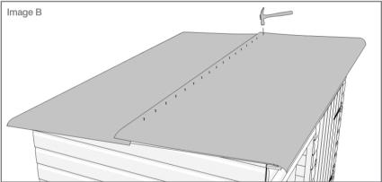
Once the felt is secure, you can cut off any excess and attach the barge boards which will hide any untidy edges. Please note only 3 bargeboards will be supplied with pent style sheds. There is no bargeboard for the lower edge to allow water to run off the roof.
