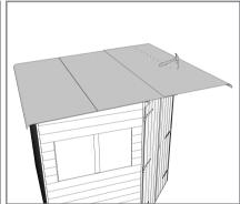
Once you have attached the felt, you can trim off any excess and then attach the barge boards as per the instructions. This will hide any untidy edges.
